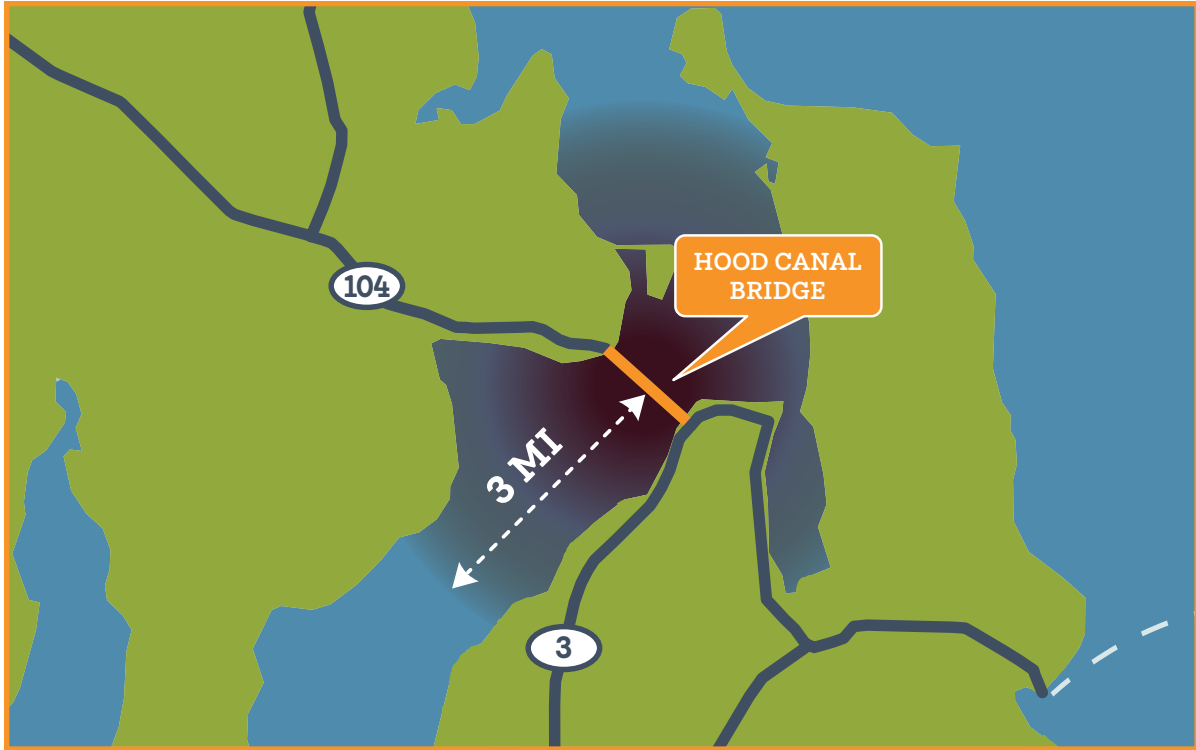
The bridge impacts temperature, currents, and salinity 65 ft below the surface and up to 3 miles away from the bridge.
