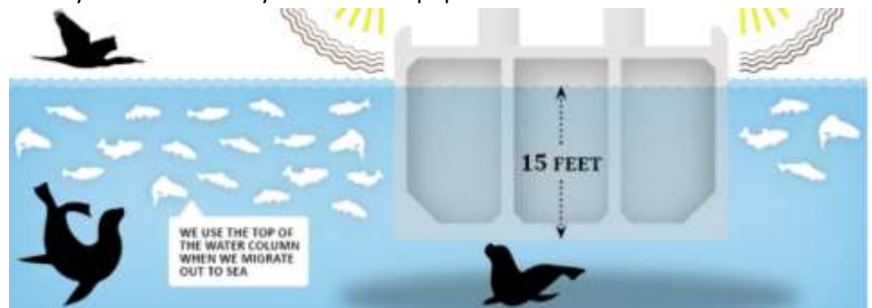
Figure 2. The bridge pontoons are a physical barrier for surface-oriented juvenile steelhead, slowing migration and increasing vulnerability to predation. Image property of LLTK.
