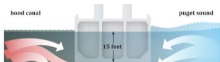
Figure 4. The bridge pontoons extend into the surface layer of the water column, impacting temperature, salinity, and currents and causing increased mixing near the bridge. Image property of Long Live the Kings.
