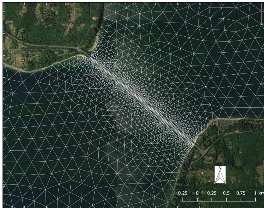
Figure 5. Salish Sea model grid with refinement in the region to facilitate incorporation of the bridge block elements. The grid size is refined such that cell centers are separated by the bridge width distance of 18.3 m. The bridge draft is represented by two layers whose combined thickness is equal to 4.57 m.
